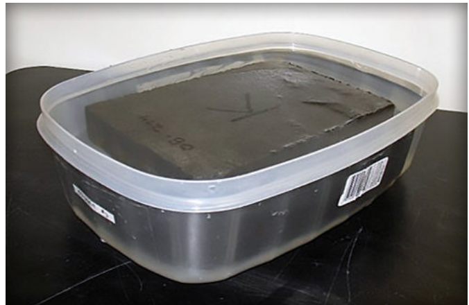
Figure 3. Test specimen from a slab immersed in a 3% saline solution ready for exposure to laboratory freeze-thaw cycles.
